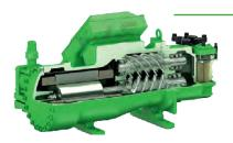
All ElectraTherm ORC systems are powered by BITZER's semi-hermetic, twin-screw expander. This allows ElectraTherm's ORC process to utilize much more variable heat sources than the leading turbine technologies. This is made possible by the expanders' ability to handle "wet" dual-phase flow leading to greater turndown ratios allowing for continuous power generation when dealing with inconsistent thermal input.
